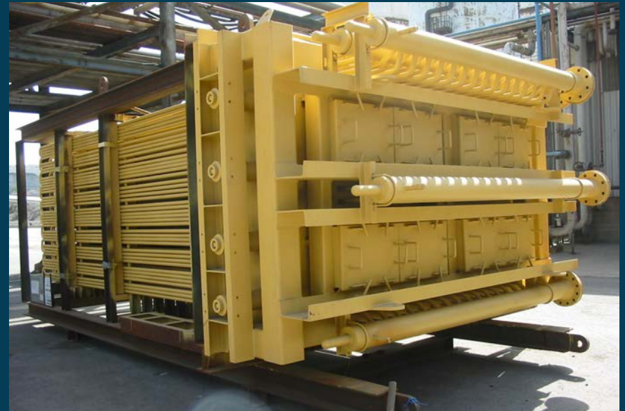
STEAM BOILER OSCHATZ-CMF superheater tube bundle dim. [mm]: 2.550 x 3.300 x 6.900 (H) weight: 20.000 kg
